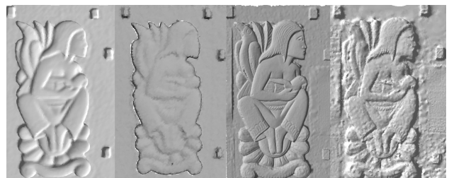
Figure 8: Visual quality check from left to right Carmine 1.09, Kinect, DCC and webcam with 123DCatch
