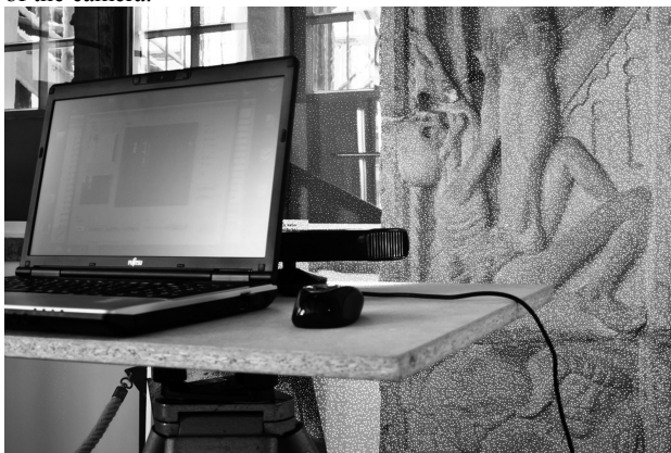
Figure 3: Infrared photo showing the point pattern and the Kinect on site in operation
