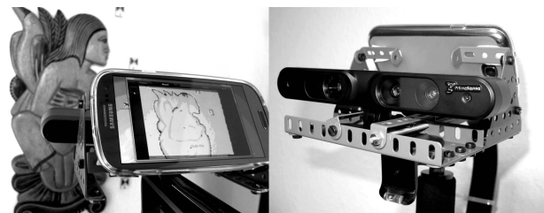
Figure 4: Primesense Carmine 1.09 mounted on a steady cam together with a smartphone as a control unit
