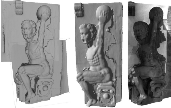
Figure 10: Alignment of two single scans. Left false colours, right textured after vertex colour transformation
