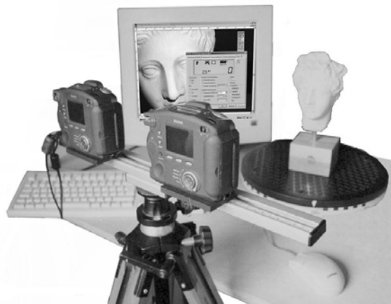
Figure 11: Computer controlled recording of image objects. Here a stereo arrangement with the object on a turntable.
