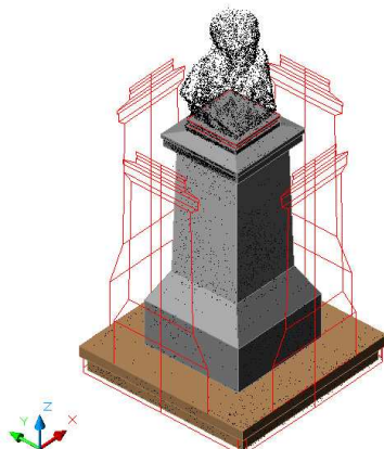
Figure 4. Construction of discrete structures over the point cloud
